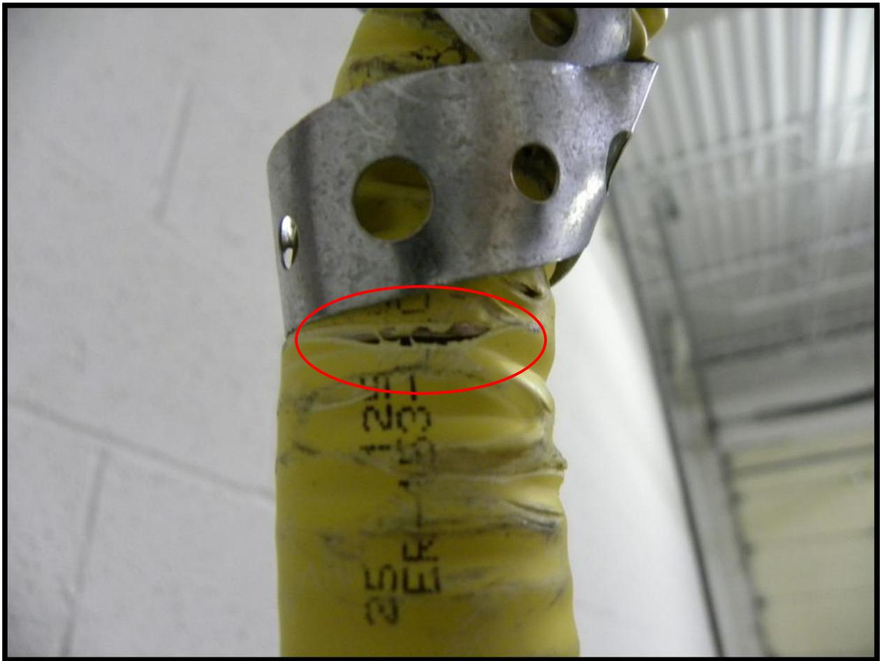
Figure 6. A perforation in the insulation resulting from the use of metal pipe straps
