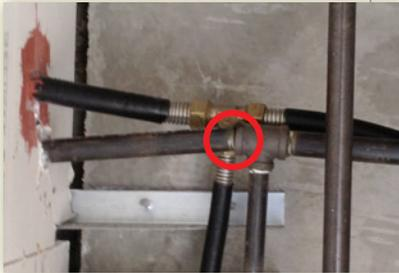
The black iron pipe, which was installed next to CounterStrike, fractured in the same test. It took 96 man hours to install the black iron pipe versus just 32 man hours to install CounterStrike.
